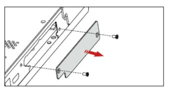
**Step 2** Insert the Wi-Fi Module into the port on the rear of the panel until firmly seated, using the 2 screws to secure it.
