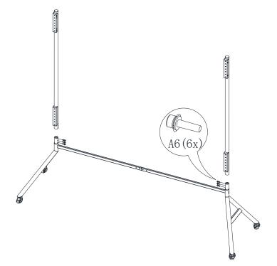
7. Connect the upper beam to the right and left castor bases, as shown below:
